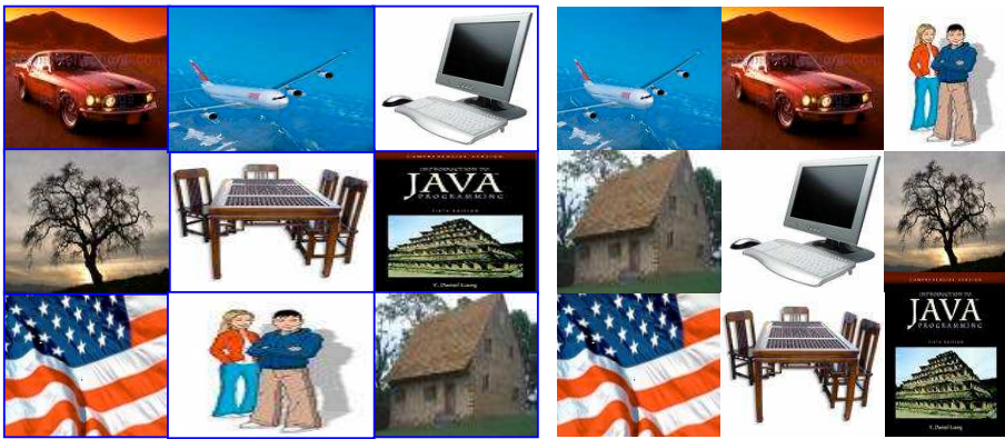
Fig. 1. The Match-n-Go login screen. Note that the password is contained in the left-hand panel of graphics. The user must locate the graphic in the password by noting the position (X,Y coordinate) on the left panel and move the corresponding graphic on the right panel to the same position. This process is repeated for each graphical element in the password.
